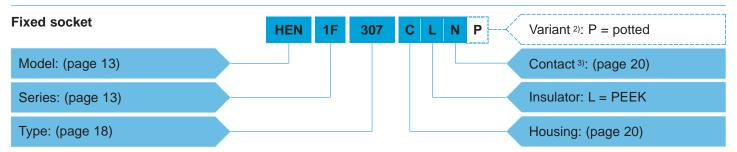
**HEN.1F.307.XLNP** = fixed socket, nut fixing, for printed circuit, key (N), (back panel mounting), watertight, 1F series, multipole with 7 contacts, chrome-plated brass outer shell, PEEK insulator, female print contacts.
