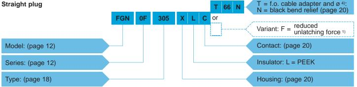
FGN.0F.305.XLC = straight plug with key (N), 0F series, multipole with 5 contacts, anthracite nickel-plated Avional outer shell, bronze latch sleeve, PEEK insulator, male crimp contacts.
