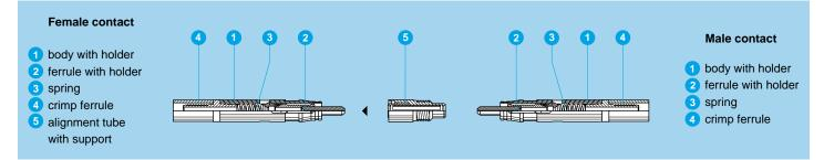
Contacts are provided in two forms: with a standard crimp barrel for large conductors (see fig. 1), or with a reduced crimp barrel for smaller conductors (see fig. 2).
