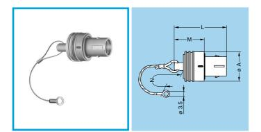
Lanyard material: Stainless steel Crimp ferrule material: Nickel-plated brass + polyolefin ĕ
